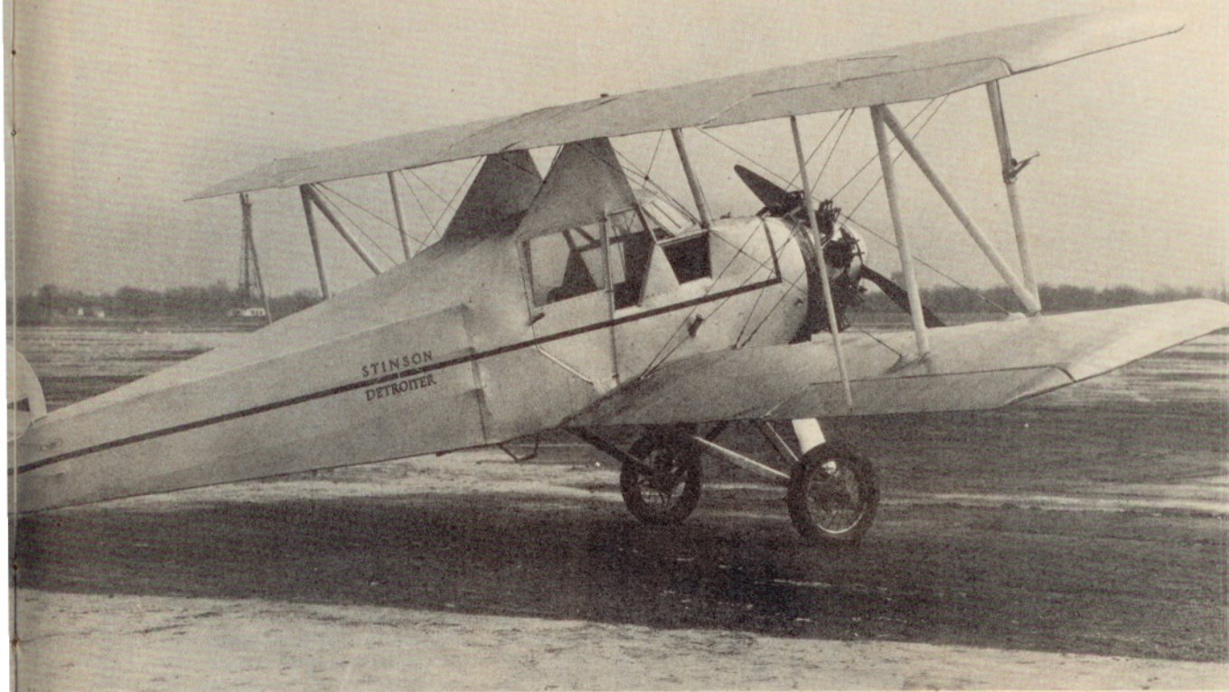
The original Stinson Detroider was anything but handsome. Notice that the cabin projects slightly above the upper longeron lines. The generous dihedral on the bottom wing contributed much to the airplane's noted stability. Ford Motor Co. photo.
